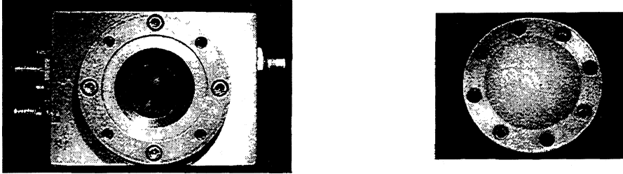
Fig. 7. Actual picture of an assembled block, with the polyethylene lens removed to show the AR coated silicon hyperhemisphere.
